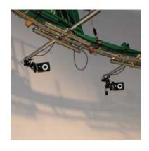
The floor dimensions are 20m(L)x13m(W)x6.6m(H) and the basic capture area is 12m(L)x8m(W)x4.5m(H) but it can be customized to an area suitable according to the contents. There are 22 Vicon T160 devices and the number of personnel doing simultaneous recording is a maximum of 6 people. They say that there is an insufficient amount of advertising to the industry even with this many motion capture studios.
